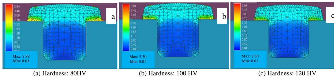
Fig. 6. Hardness equivalent strain profile of different materials.
