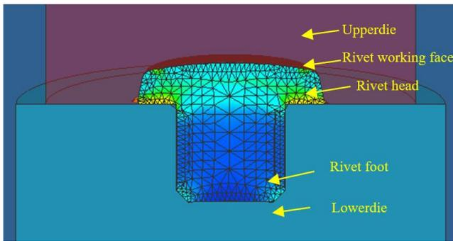
Fig. 1. Simplified cold forming model.
