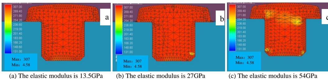
Fig. 5. Equivalent strain profile of rivet forming under different elastic modulus.
