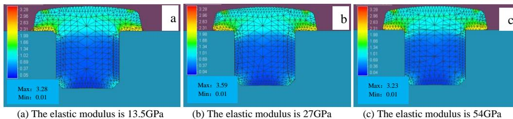
Fig. 4. Equivalent strain profile of rivet forming under different elastic modulus.
