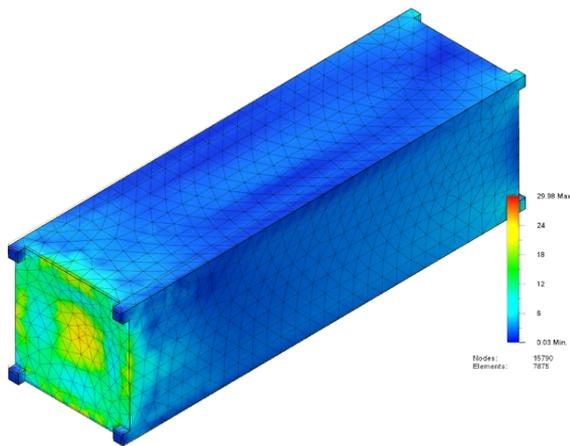
Fig. 9. Static strain in Fusion360.
