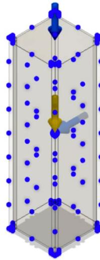
Fig. 5. Location of the applied forces in Fusion 360.
