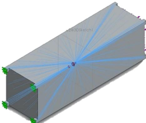
Fig. 4. Location of the applied forces in SolidWorks.
