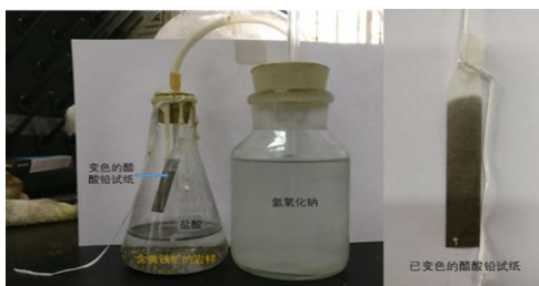
Fig. 2. Experimental diagram of H 2 S secondary gas detection by lead acetate test paper.
