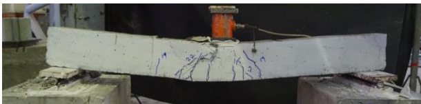
Fig. 8. Failure mode of beam control.
