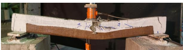
Fig. 9. Failure mode of beam JFRP-A.
