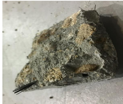
Fig. 8. A photo of a fractured concrete cylinder showing exposed fibers.
