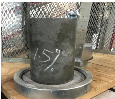
Fig. 3. A cylindrical concrete mold labeled according to its percentage carbon fiber composition.
