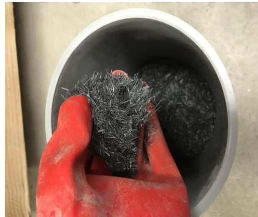
Fig. 1. A photo of the recycled carbon fibers used in the concrete mixes.
