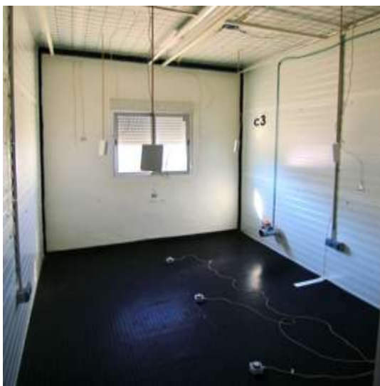
Fig. 5. Inner view of the test cell with lux meter distribution.
