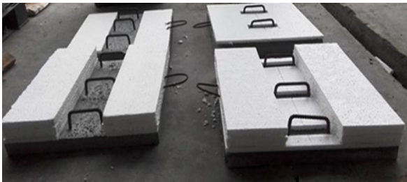
Fig. 1. Staggered shear connectors positioned on both concrete layers.
