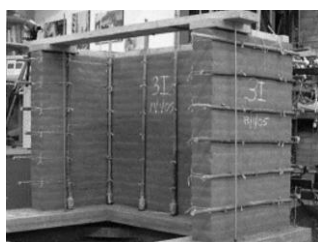
Fig. 18. Application of external bamboo.
