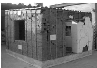
Fig. 17. Cane external reinforcement
