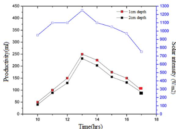
Fig. 4. Productivity of solar distiller without modifications
