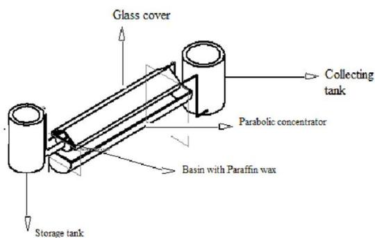
Fig. 1. Schematic diagram of solar concentrated distiller
