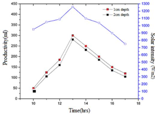
Fig. 6. Productivity of solar distiller with trays
