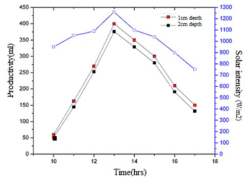
Fig. 11. productivity of paraffin wax distiller with mild steel billets
