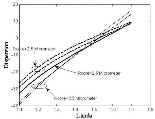
Fig. 5. Dispersion vs. Landa (wavelength) ( $\mu\text{m}$ )  $n_1 = 1.5, n_2 = 1.4953$
