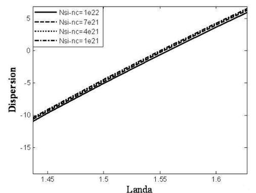
Fig. 8. Dispersion vs. Landa (wavelength) ( $\mu\text{m}$ )
