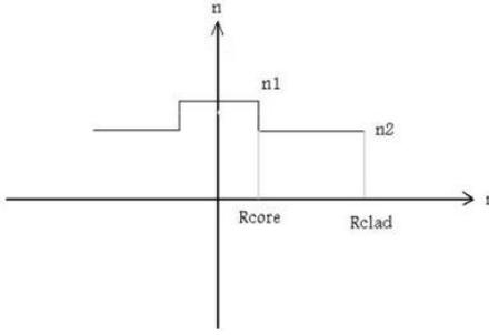
Fig. 1. Profile of step index traditional fiber.
