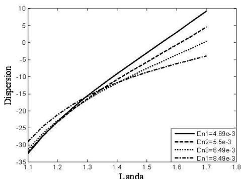
Fig. 4. Dispersion vs. Landa (wavelength) ( $\mu\text{m}$ )  $R_{\text{core}} = 2.5 \mu\text{m}, Dn = n_1 - n_2$
