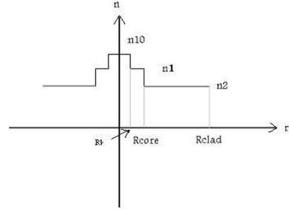
Fig. 2. Homogenous profile of Si-Nc and Er doped fiber
