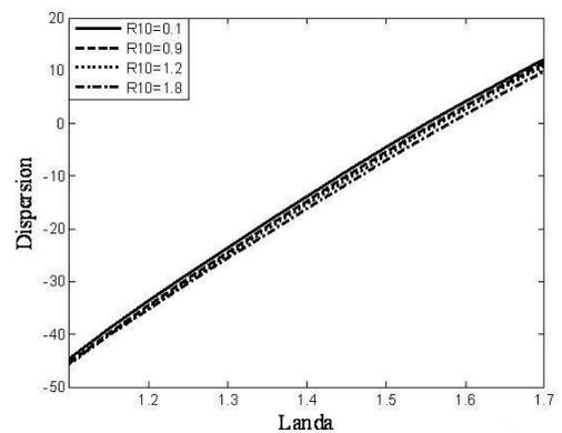
Fig. 7. Dispersion vs. Landa (wavelength) ( $\mu\text{m}$ )
