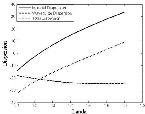
Fig. 3. Dispersion Vs. Landa (wavelength) ( $\mu\text{m}$ )
