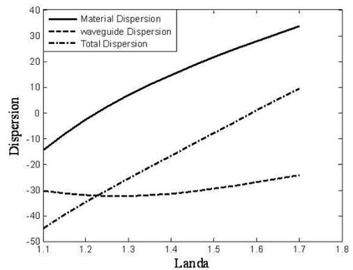
Fig. 6. Dispersion vs. Landa (wavelength) ( $\mu\text{m}$ )
