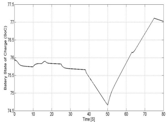
Fig. 9. Battery state of charge with respect to the current
