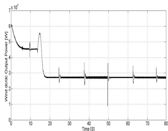
Fig. 5. Power delivered to the dc link from wind turbine
