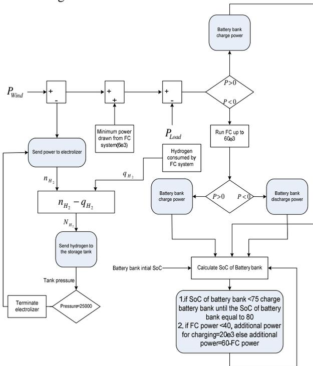
Fig. 3. The overall algorithm used in the main controller
