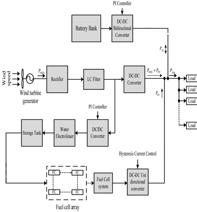
Fig. 1. Overall system configuration
