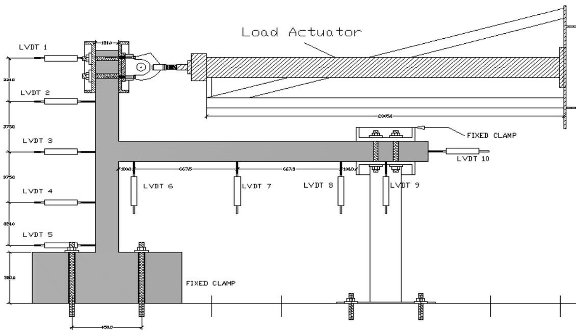
Fig. 1. Sample of wall-slab connection together with positions of LVDT's
