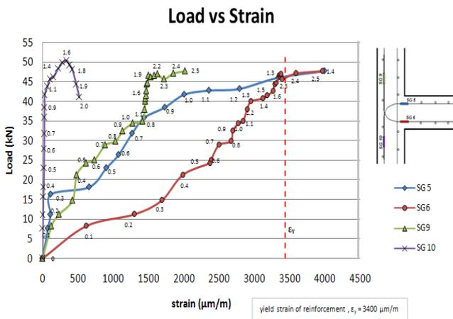
Fig. 14. Load versus strain for reinforcement.
