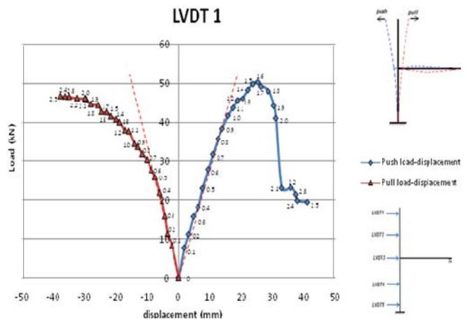
Fig. 13. Load-displacement profile of wall (LVDT 1)
