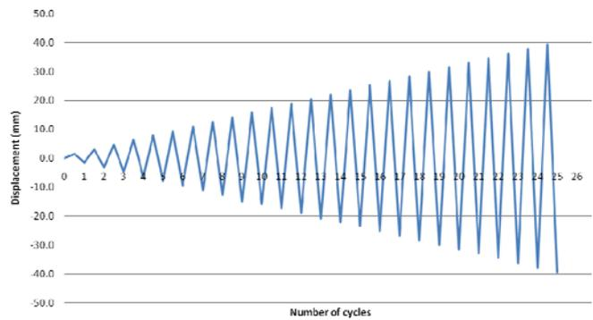
Fig. 9. Loading regime for the testing procedure.
