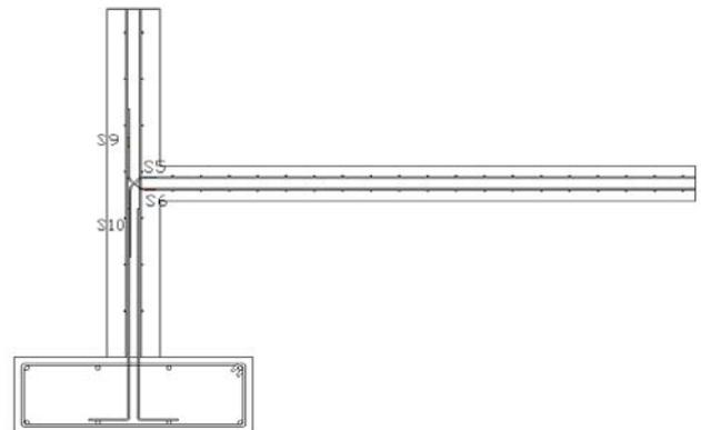
Fig. 8. Location of strain-gauge on the BRC-A7
