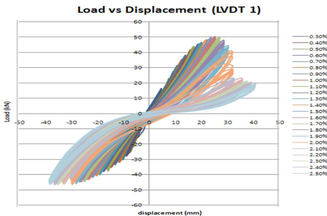
Fig. 15. Hysteresis loops of wall based on LVDT 1
