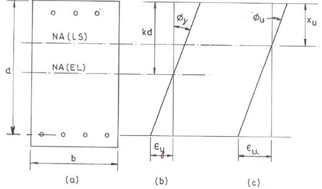
Fig. 2. (a) Cross section of wall, (b) Strain at yield state, (c) Strain at ultimate state
