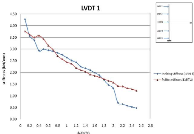
Fig. 16. Stiffness profile of wall based on LVDT 1.
