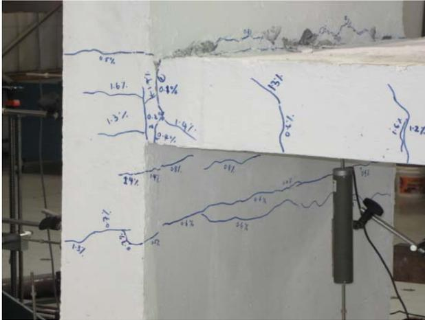
Fig.10: Cracks occurred wall-slab joint from side view.
