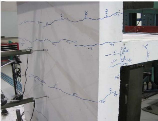
Fig. 11. Cracks at wall-slab joint from rear view.
