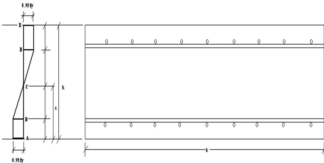
Fig. 3. Stress diagram of wall section.
