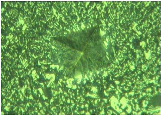
Fig. 13. Microstructure of Cobalarc-9 weld layer on mild steel 0.57mm away from weld fusion line at 400X Magnification
