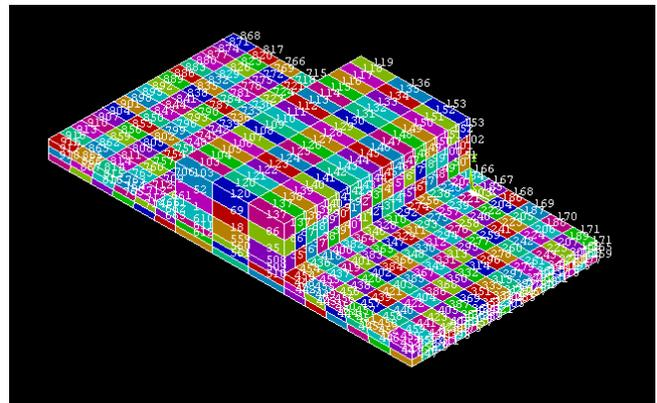
Fig. 5. Meshed 5mm thick MS model with three Cobalarc layers of 4mm thickness each
