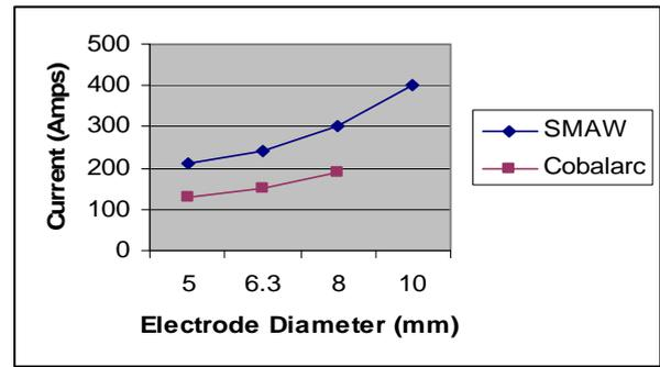
Fig. 2. Low amperage of Cobalarc
