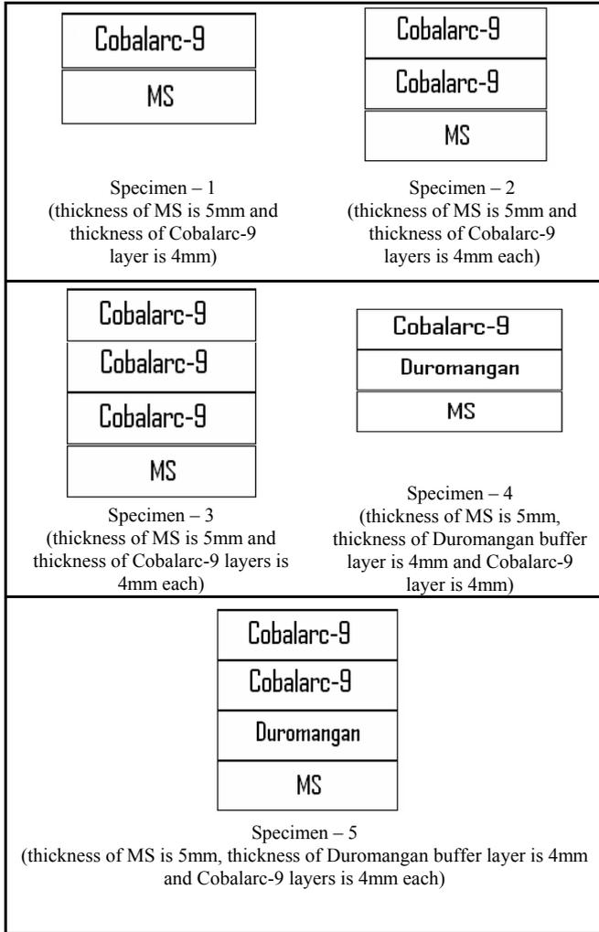
Fig. 3. Layout of five specimens prepared by hardfacing
