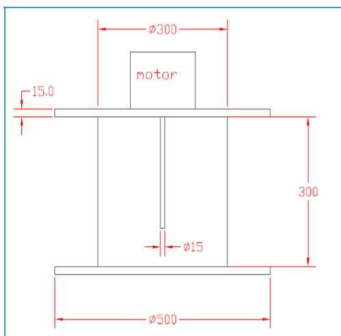
Fig. 6. Schematic diagram of sand slurry wear tester
