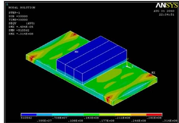
Fig. 10. Von Mises residual stress plot for 5mm thk plate (preheat 473K) with three Cobalarc hardfacing layers of 4mm thk each
