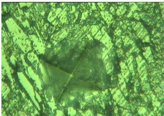
Fig. 15. Microstructure of cobalarc-9 weld layer on mild steel 3.0 mm away from weld fusion line at 400X Magnification
