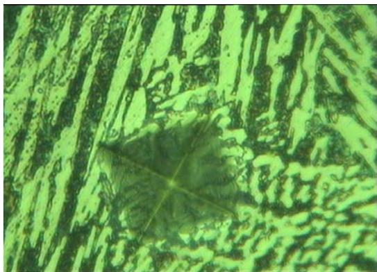
Fig. 14. Microstructure of Cobalarc-9 weld layer on mild steel 1.55mm away from weld fusion line at 400X Magnification
