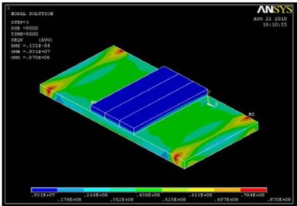
Fig. 8. Von Mises residual stress plot for 5mm thk plate (preheat 303K) with one Cobalarc hardfacing layer of 4mm thk
