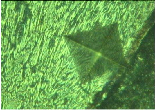
Fig. 12. Microstructure of Cobalarc-9 weld layer on mild steel at weld fusion line at 400X Magnification
