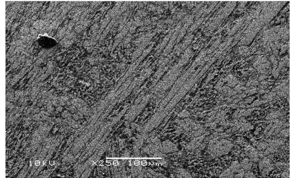
Fig. 22. Scanning Electron Microstructure of Cobalarc-9 weld layer showing the  $M_7C_3$  carbides (250X)
