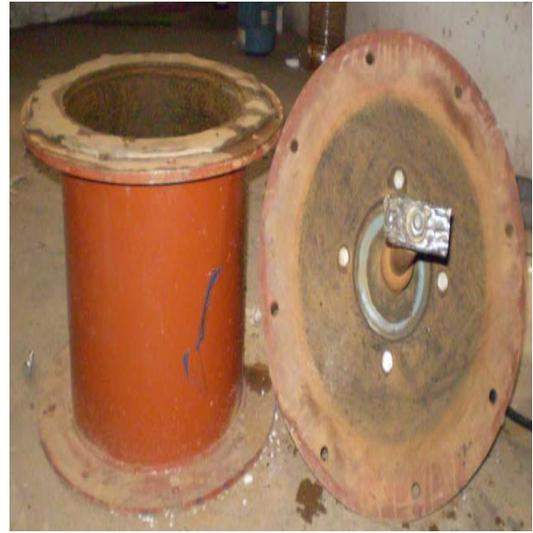
Fig. 7. Sand Slurry wear tester
