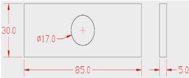
Fig. 1. Mild Steel specimen for slurry test
