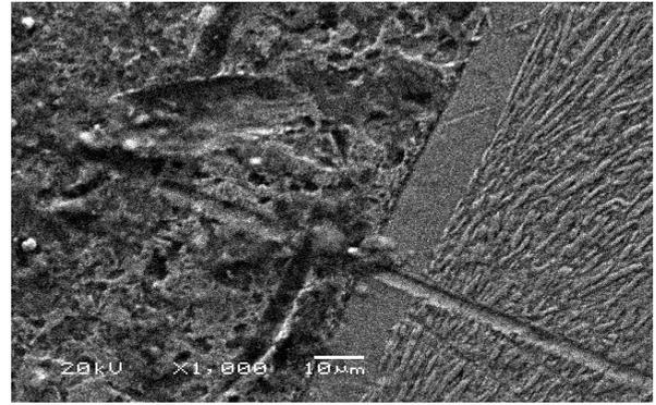
Fig. 21. Scanning Electron Microstructure of base metal (mild steel) and Cobalarc-9 weld layer showing the weld fusion line (1000X)
