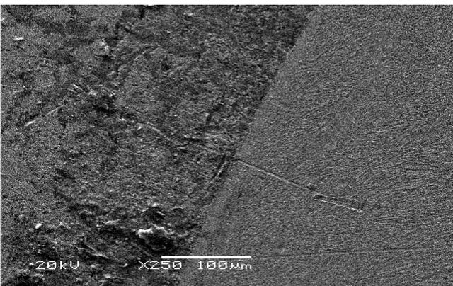
Fig. 20. Scanning Electron Microstructure of base metal (mild steel) and Cobalarc-9 weld layer showing the weld fusion line (250X)
