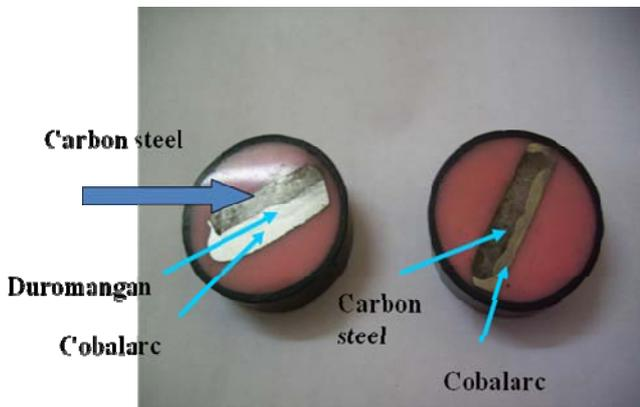
Fig. 4. Actual specimens prepared by hardfacing for microstructure / microhardness analysis
