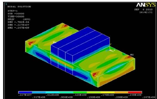
Fig. 11. Von Mises residual stress plot for 15mm thk plate (preheat 473K) with three Cobalarc hardfacing layers of 4mm thk each
