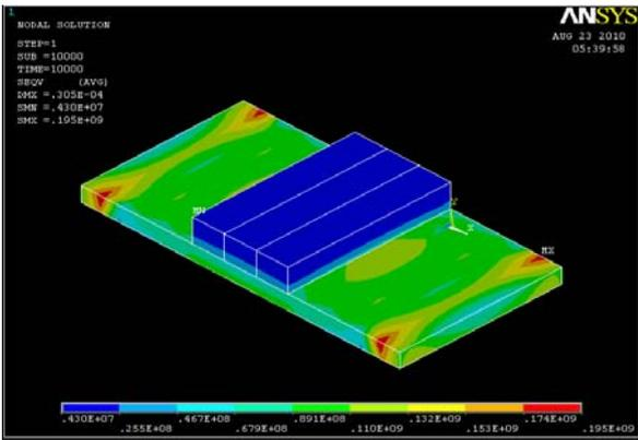
Fig. 9. Von Mises residual stress plot for 5mm thk plate (preheat 303K) with two Cobalarc hardfacing layers of 4mm thk each
