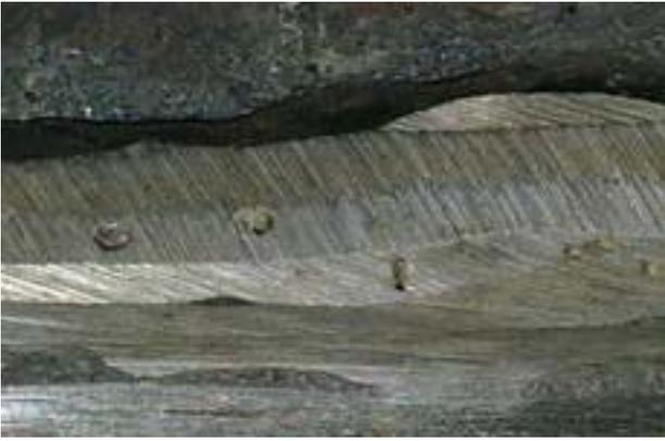
Fig. 18. Absence of cracks in 16mm thick mild steel welded with tubular electrode producing a austenitic matrix
