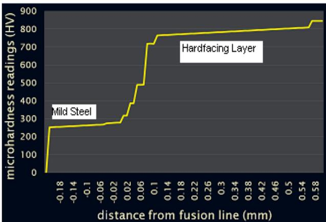
Fig. 19. Variation of hardness with distance from fusion line on Cobalarc-9 layer
