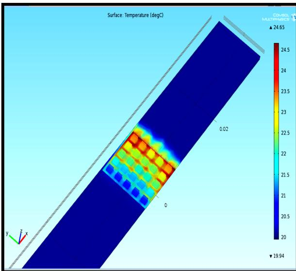
Fig. 11. 3D Temperature distribution for 2D rectangular fin array
