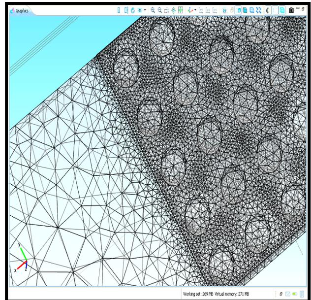
Fig. 8. 3D Mesh generation at fin assembly
