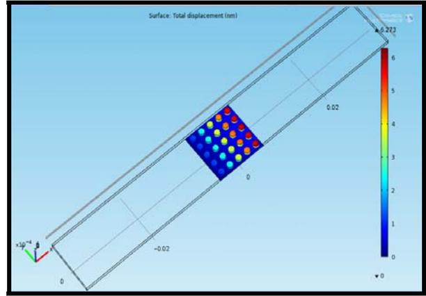
Fig. 23. thermal expansion of circular fin array
