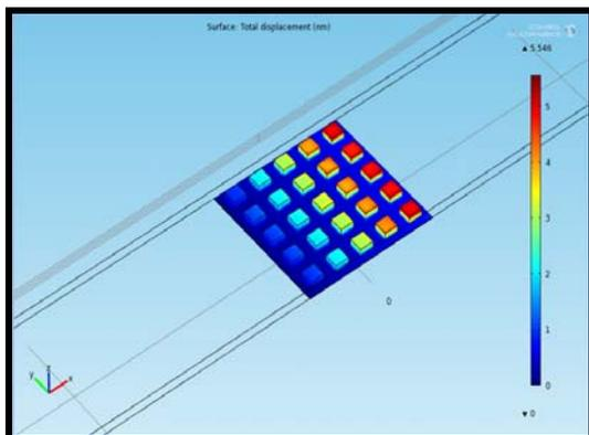
Fig. 22. Thermal expansion of rectangular fin array
