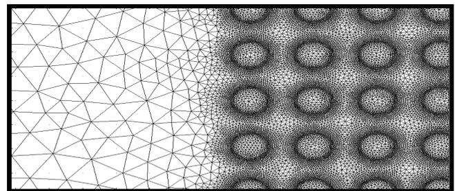
Fig. 9. 2D Mesh generation at fin assembly
