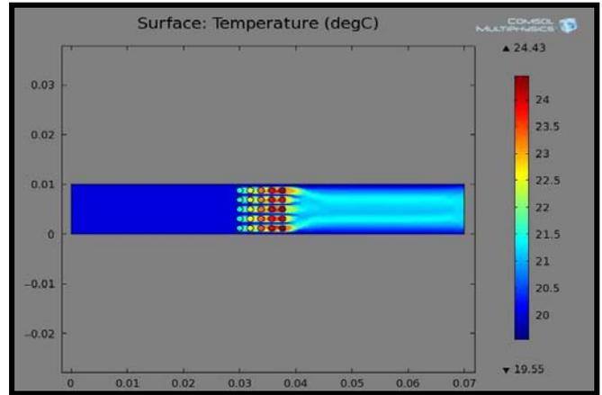
Fig. 13. 2D Temperature distribution for 2D circular fin array
