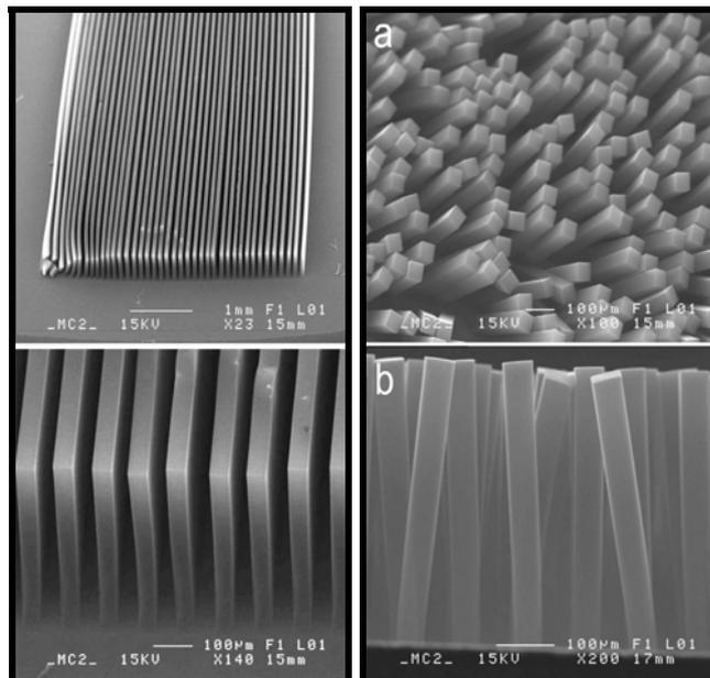
Fig. 4. SEM picture of CNT with one and two dimensional array [5].
