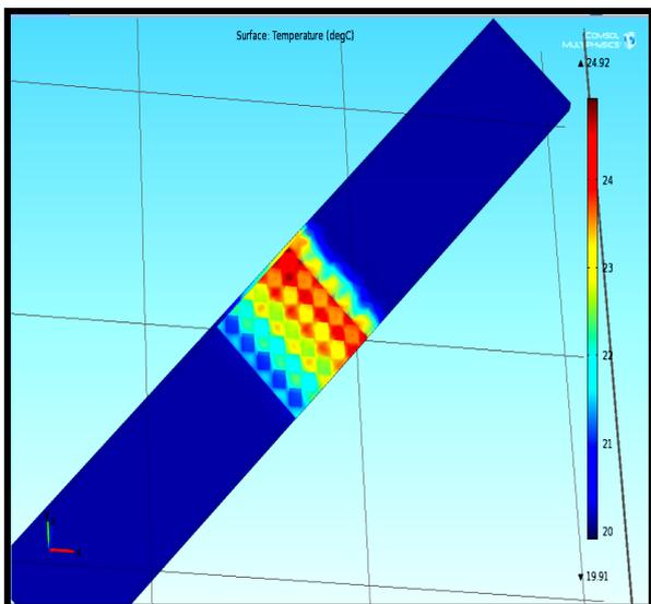
Fig. 12. 3D Temperature distribution for 2D rectangular fin array with 45 degree orientation with the flow
