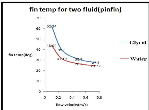
Fig.18. Comparison graph for the effectiveness of different fluids.
