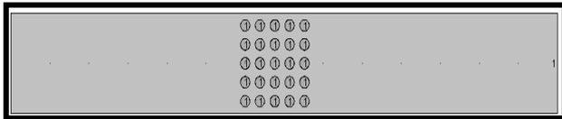
Fig. 6. 2D computational model for circular pin fin heat sink
