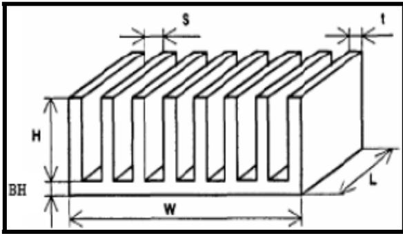
Fig. 5. Parallel plate heat sink showing all the dimensions
