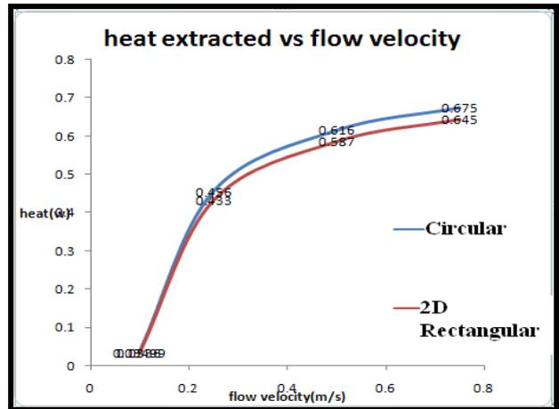
Fig.19. Heat extraction graph for rectangular and circular fin array
