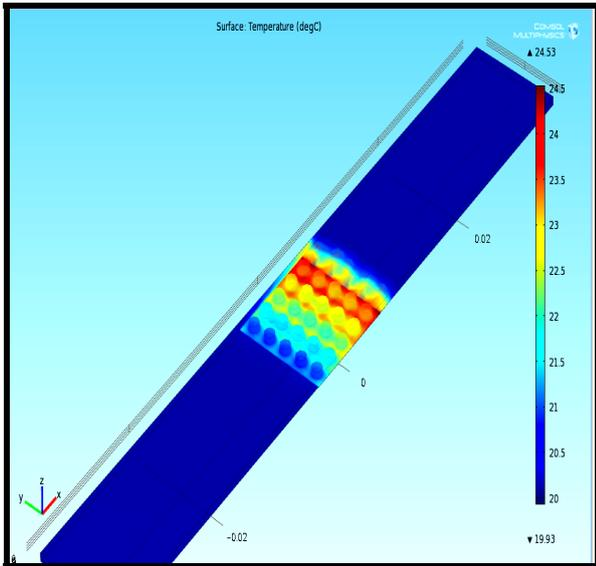
Fig. 10. 3D Temperature distribution for 2D circular fin array
