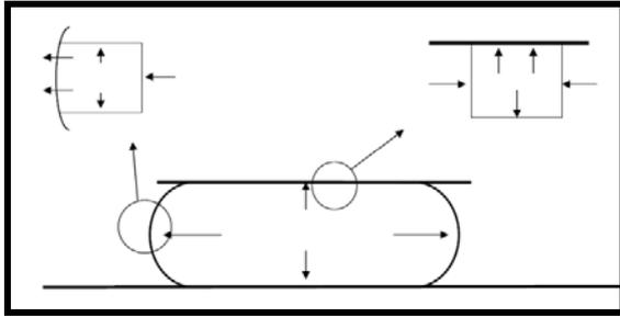
Fig. 20. Thermal expansion of adhesive bond
