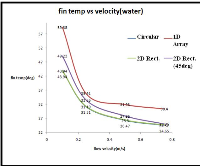
Fig.17. Fin temperature vs. Velocity for different fin geometry for water
