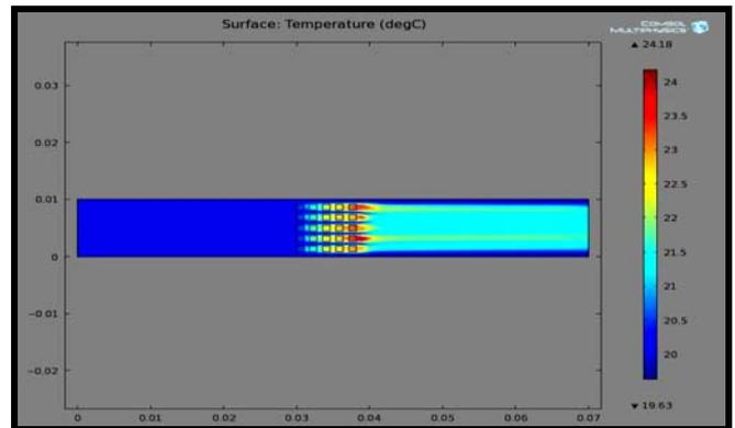
Fig. 14. 2D Temperature distribution for 2D rectangular fin array
