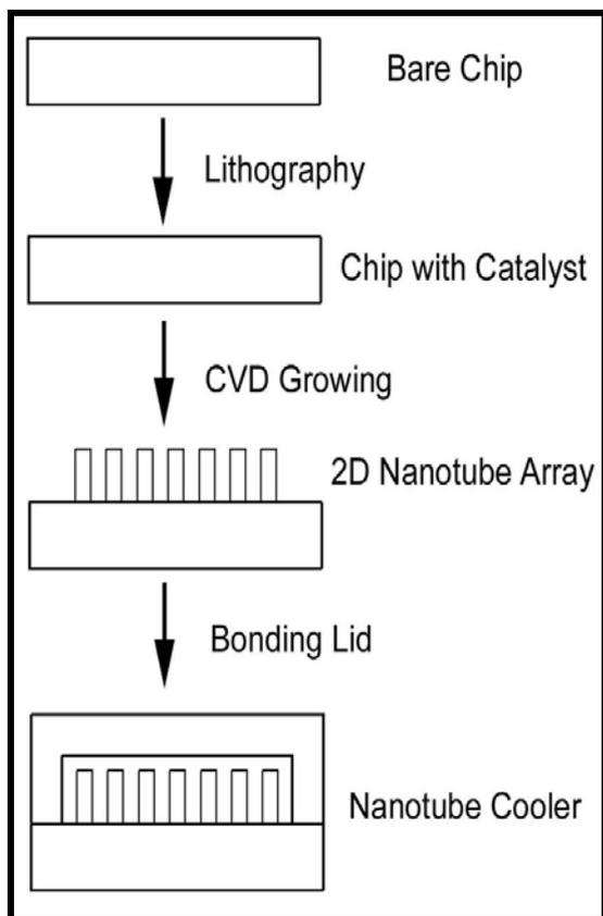
Fig.3. Process to manufacture CNT based micro-cooler
