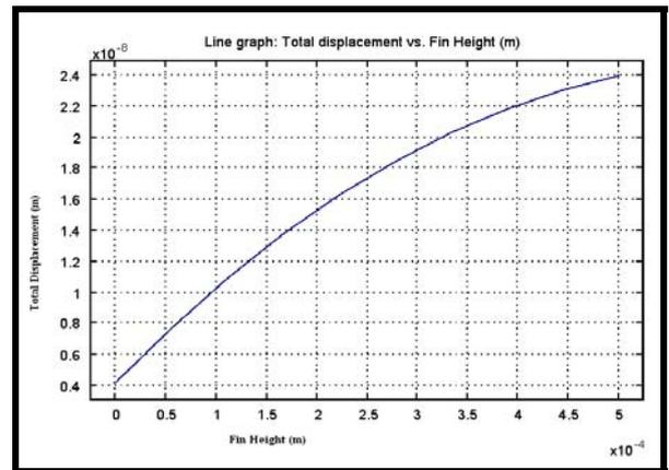
Fig. 24. Total displacement curve along the fin height for circular fin array.
