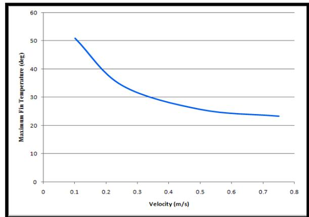
Fig. 15. Maximum fin temperature Vs. Velocity graph.
