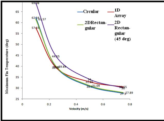
Fig.16. Fin temperature Vs. Velocity for Different fin geometry for glycol
