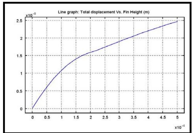
Fig. 25. Total displacement curve along the fin height for rectangular fin array.
