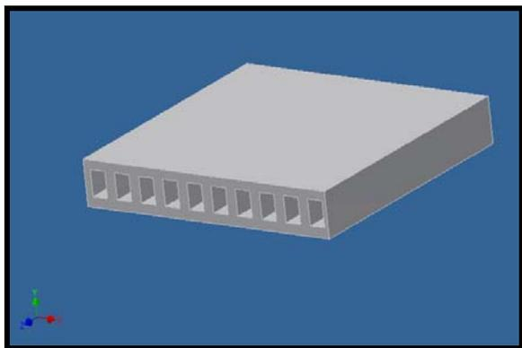
Fig.2. Micro-channel cooler
