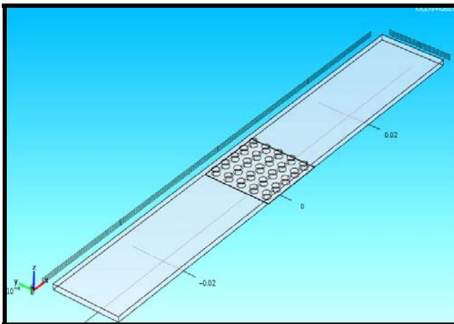
Fig. 7. 3D computational model for circular pin-fin heat sink
