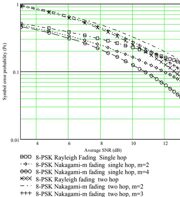
Fig. 3 Comparison of performance of single and dual hop fading channel for 8-PSK scheme.
