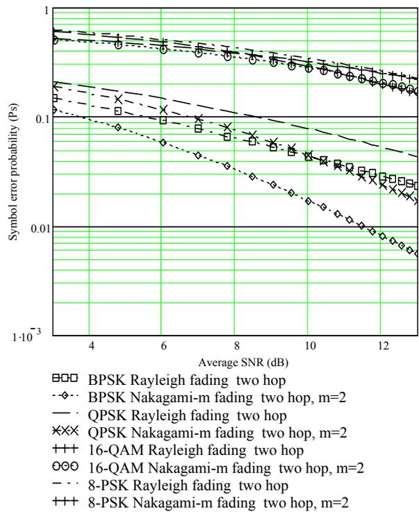
Fig. 5 Comparison of modulation scheme on two hop link.
