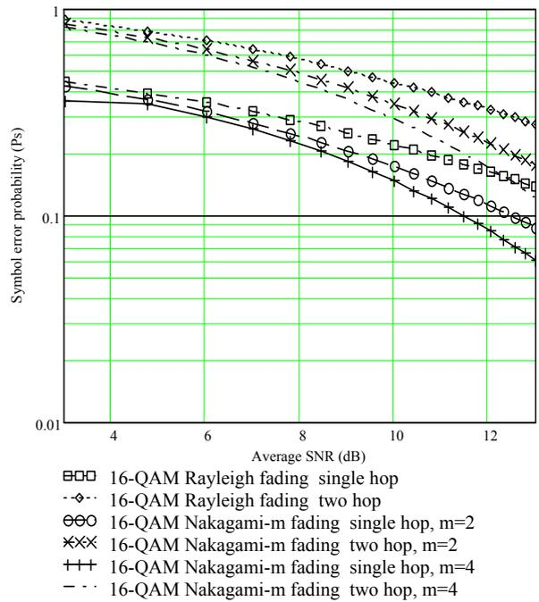
Fig. 4 Comparison of performance of single and dual hop fading channel for 16-QAM scheme.
