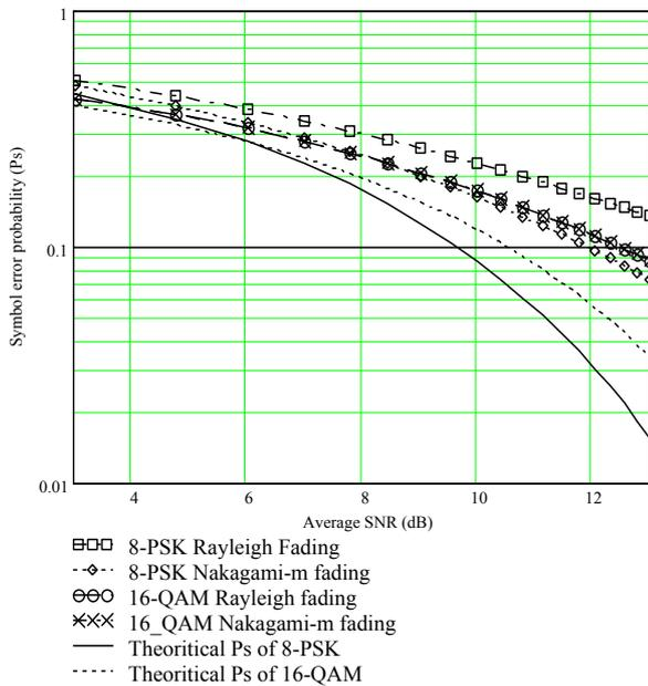
Fig. 2 Comparison of theoretical SER and SER of fading channel for single hop wireless link.
