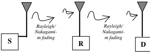
Fig. 1 Two-hop wireless link.
