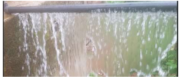
Fig. 1. Photo of water curtain switched on during experiment.
