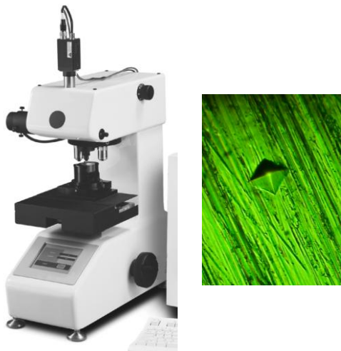
Fig. 10. Hardness tester FM-700 (Future-tech Corp, Tokyo, Japan) and sample image during knife testing.
