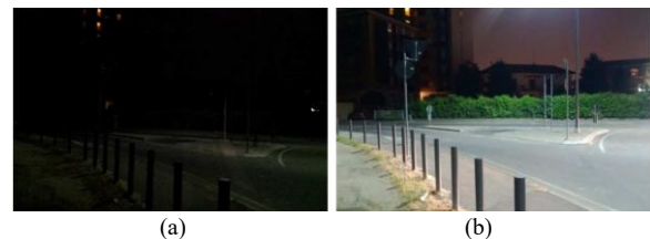
Fig. 2. OIS OFF (a) vs. OIS ON (b) in an outdoor night picture [1].
