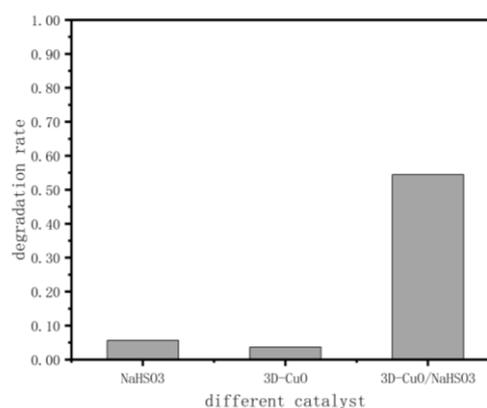
Fig. 1. The degradation effects of MO with the different catalysts under the optimized experimental conditions.
