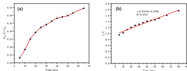
Fig. 3. (a)The degradation curve of MO under the optimized condition; (b)Ln(C/C0)-irradiation time curve.
