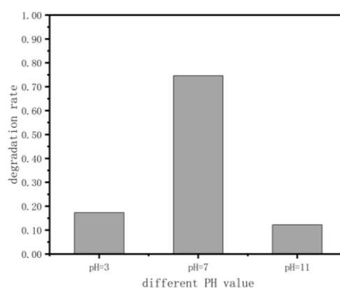
Fig. 2. Effect of pH value on the degradation rate of MO in 3D-CuO / NaHSO<sub>3</sub> system.
