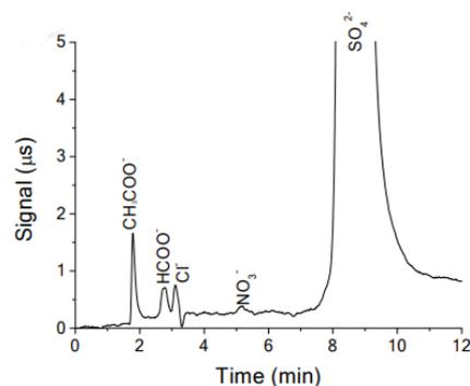
Fig. 4. The degradation products of MO by the ion chromatography.
