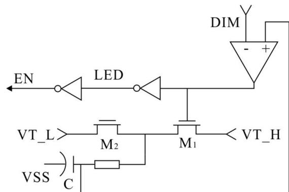
Fig. 2. Analog dimming PWM signal equivalent circuit diagram.
