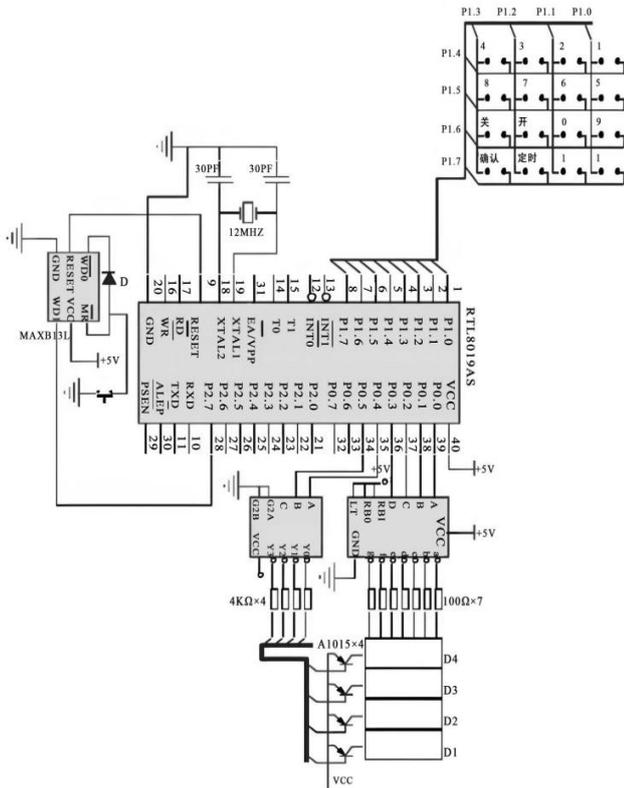
Fig. 1. Integrated circuit structure of ARM RTL8019AS host controller.
