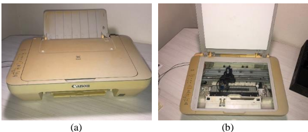
Fig. 2. (a) Printer casing; (b) Internal observation panel of the printer.
