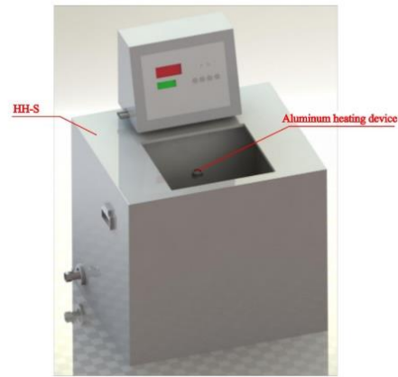
Fig. 2. Schematic diagram of heating device.
