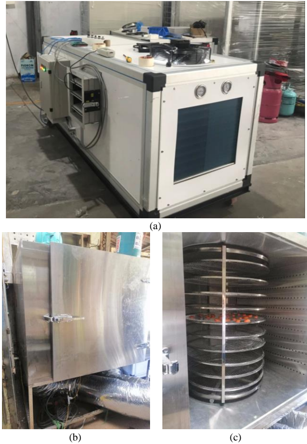
Fig. 1. The heat pump system (a), the drying chamber (b), and trays (c) fabricated in this project.
