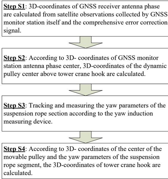
Fig. 1. Flowchart of the GNSS method.
