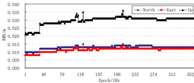
Fig. 8. RMS of the monitor station in North, East and Up directions.
