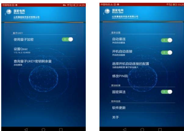
(a) Applying the quantum encryption (b) Basic configuration and algorithm Fig. 11. Service configuration of mobile terminals.
