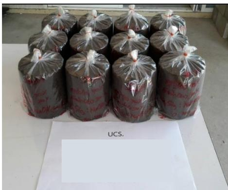
Fig. 3. MLS-BA geopolymer specimens.
