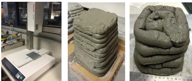
Fig. 1. Laboratory-scale gantry type 3D printer and 3D-printed block specimens using different nozzle diameters.
