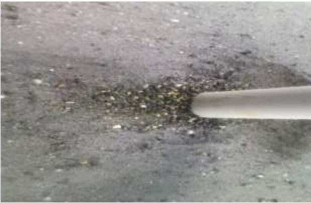
Fig. 3. Secondary armour layer formed around a pier in the laboratory flume.
