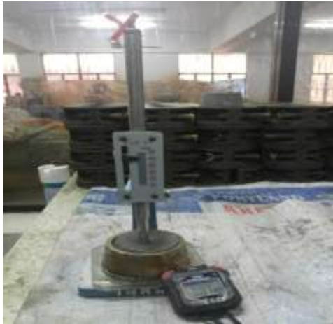
Fig. 1. Consistency test in the BUET lab.
