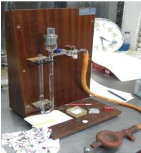
Fig. 6. Blaine air-permeability apparatus in BUET laboratory.
