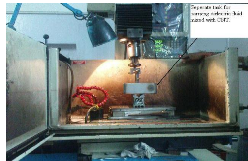
Fig 5. EDM set up using SWCNT
