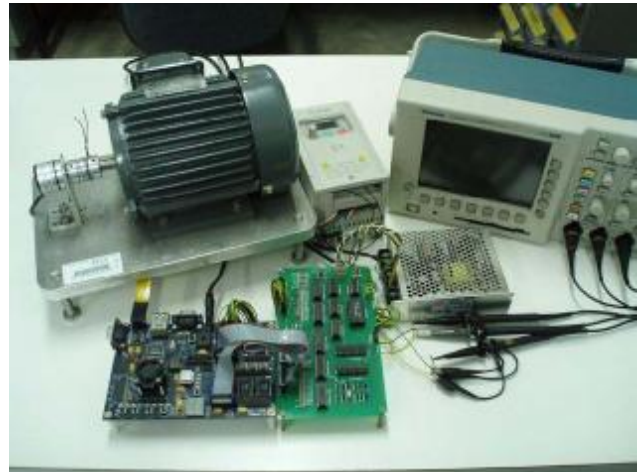
Fig. 28: FPGA-Based Induction Motor Smart Control System Experiment Environment [42].
