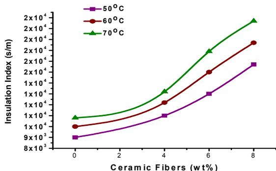
Fig. 4c. Insulation indexes at diverse ceramic fiber loadings in the rubber matrix
