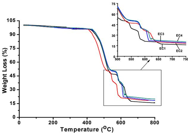
Fig. 9a. The effect of ceramic fibers concentration on the thermal decomposition of the CerF/EPDM composites
