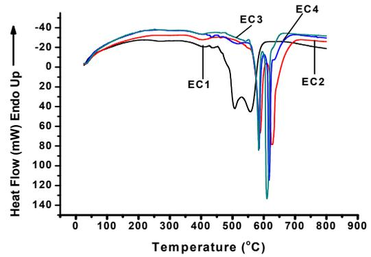
Fig. 9b. The effect of ceramic fibers concentration on the heat flow response of CerF/EPDM composites
