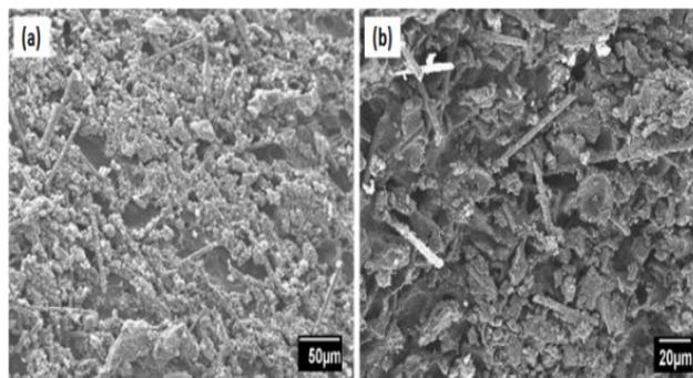
Fig. 5(a, b). Voids formation during ablation, polymer pyrolysis, char reinforcement interaction and distributed ceramic fibers in the EC4 ablated specimen
