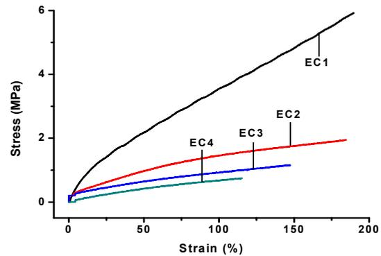
Fig. 10a. Stress-Strain contours of the fabricated CerF/EPDM composites
