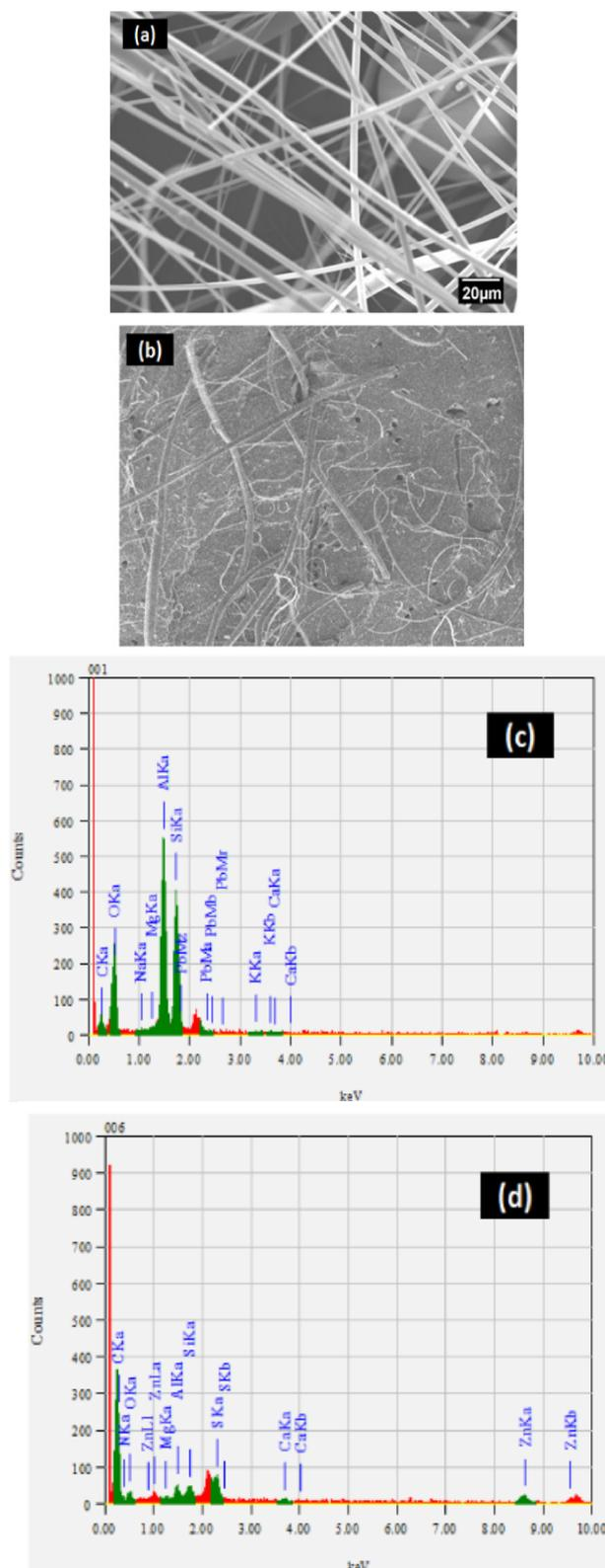
Fig. 3. SEM/EDS analyses of ceramic fibers (a, c) and 8 wt% CFs loaded composite specimen (b, d)
