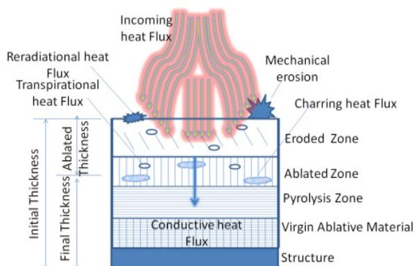
Fig. 1. Schematic illustration of the ablation mechanism of the rubber ablative composite
