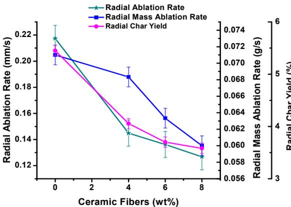
Fig. 8. Radial/mass ablation rates of the ablative composites at different CerFs concentrations in the polymer matrix
