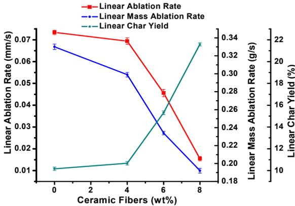
Fig. 7. Linear/mass ablation rates of the ablative composites at different CerFs concentrations in the polymer matrix
