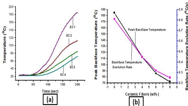
Fig. 4. Time-temperature profile (a) and peak backface temperature/backface temperature evolution rate (b) of CerF/EPDM composite
