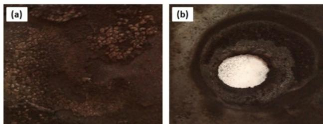
Fig. 6. Post burnt linear (a) radial (b) CerF/EPDM ablative composites
