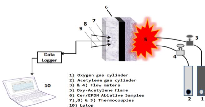
Fig. 2. Experimental setup of ablation testing of the elastomeric ablative composites
