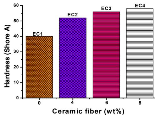
Fig. 10b. Variation in shore A hardness of the composite specimens at diverse loadings of ceramic fibers in the rubber matrix
