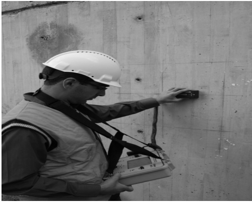
Fig. 2. Application of rebar locator device on concrete bridge pier wall.
