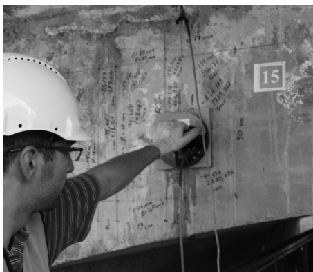
Fig. 5. Application of reinforcement corrosion resistivity (corrosion rate) device on a reinforced concrete bridge girder.
