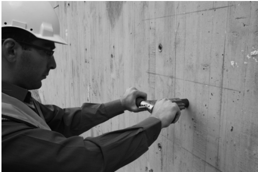
Fig. 3. Application of pin device on concrete bridge pier wall.
