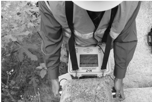
Fig. 4. Application of ultrasound pulse velocity device on a concrete bridge wing wall.
