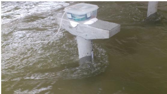
Fig. 11. While scouring (piers buried for 49 cm)
