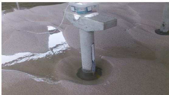
Fig. 12. After scouring (piers buried for 49 cm)
