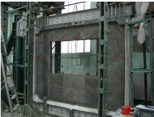
Fig. 2. Glass fiber grid and punctual anchorage application
