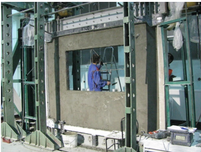
Fig. 3. Second layer of mortar application
