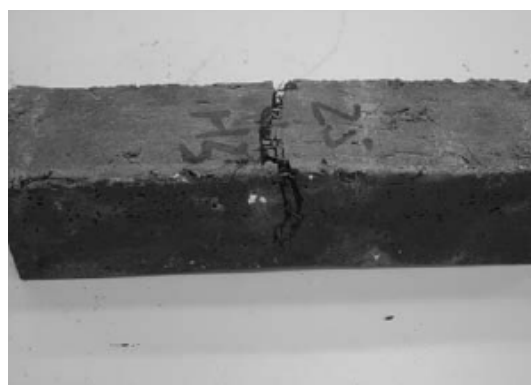
Fig. 2. Photo prism UHPC2.5 after flexural test of crack extension and failure
