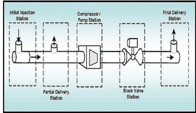
Fig. 2. A pipeline schematic [5].
