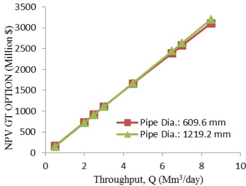
Fig. 6. NPV against gas flow rate for varying pipe sizes.
