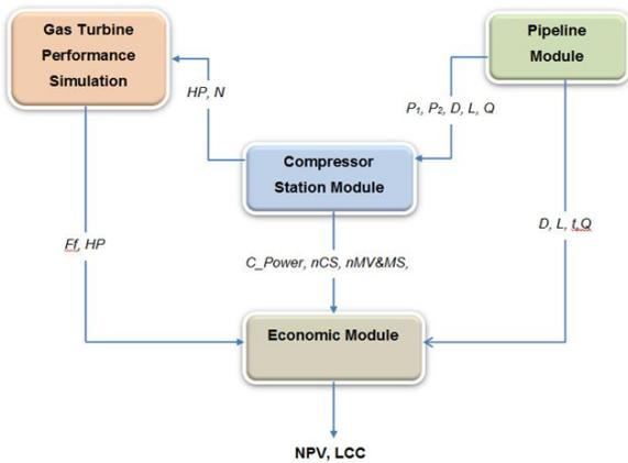
Fig. 3. Integrated techno-economic modules for gas pipeline
