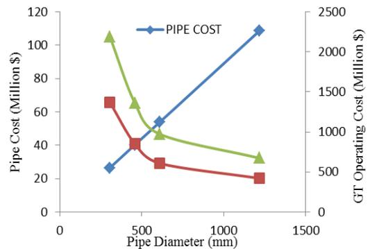
Fig. 5. GT operating cost and pipe cost variation with pipe diameter
