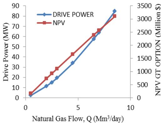
Fig. 7. Drive power and NPV against gas throughput
