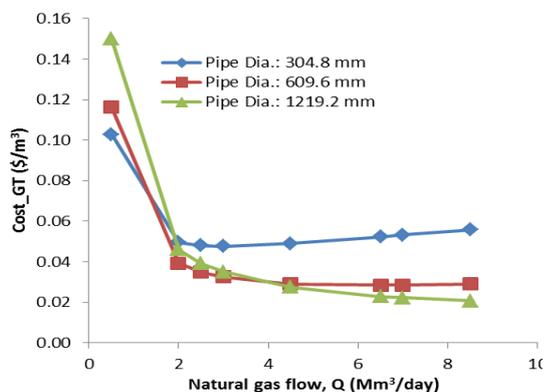
Fig. 11. Transportation cost per unit of gas against throughput for varying pipe sizes
