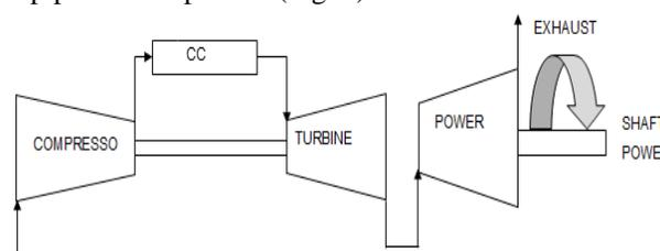
Fig. 1. Gas turbine configuration for natural gas pipeline.
