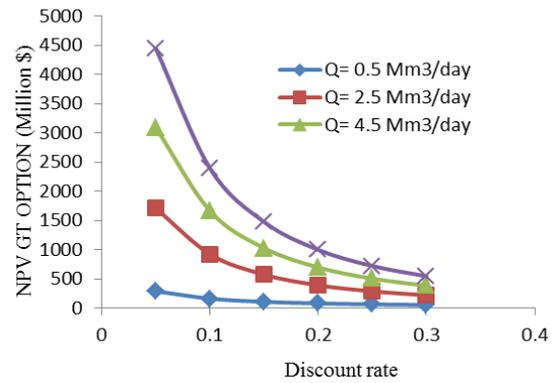
Fig. 8. NPV against discount rate for varying throughput
