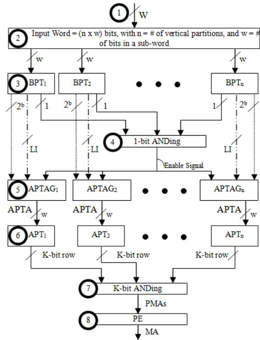
Fig. 2. Memory architecture of VP SRAM-based TCAM.
