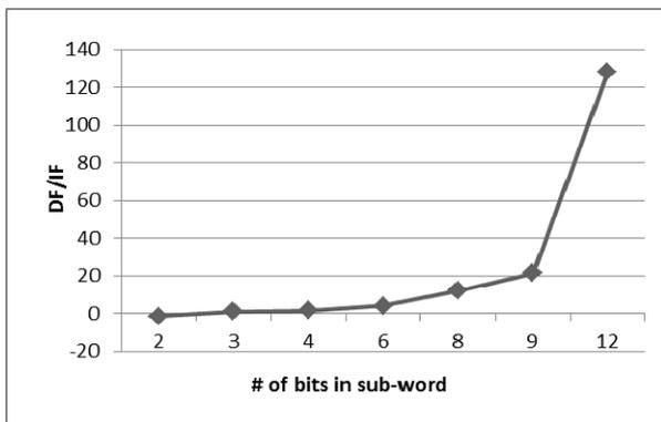
Fig. 6. This graph shows an exponential increase in the memory size of VP SRAM-based TCAM when # of bits in sub-word 'w' increases.
