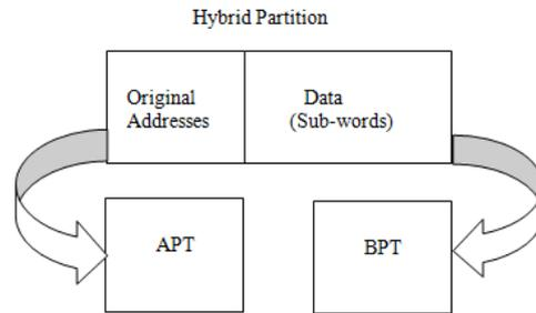
Fig. 5. Mapping of original addresses to their corresponding bits in APT and mapping of sub-words to their corresponding bits in BPT
