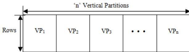
Fig. 1. Conceptual view of vertical partitioning.
