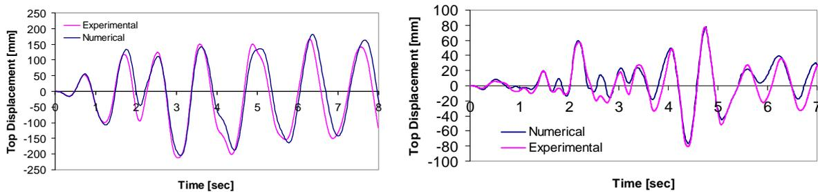
Fig. 2. Top displacement time history response of the bare structure (left) and of the fully infilled structure (right) under high-level earthquake: experimental and numerical results.
