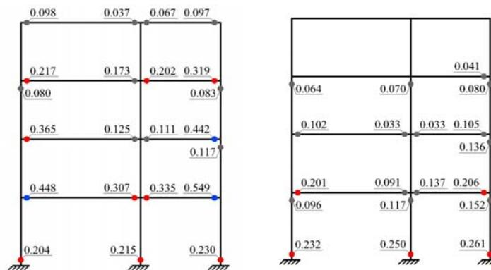
Fig. 3. Damage distribution on the external frame of the RC structure: Bare (left) and infilled (right) configurations.
