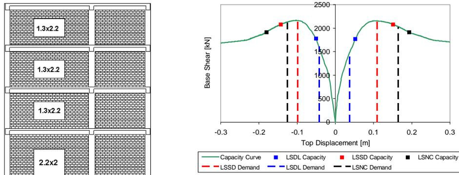
Fig. 5. Elevation view of the infilled structure with openings (left) and displacement capacity and demand for the infilled structure with openings at the different limit states (right).
