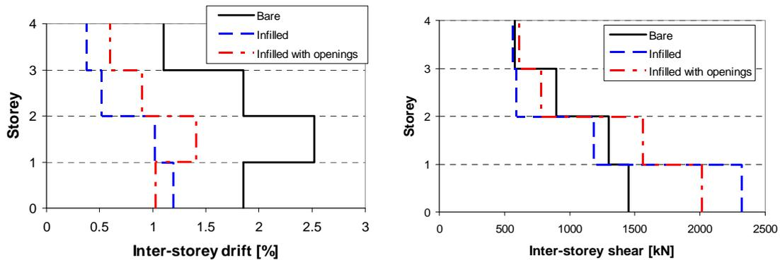
Fig. 6. Storey drift (left) and storey shear (right) profiles for the investigated structures at 0.6g seismic intensity level.
