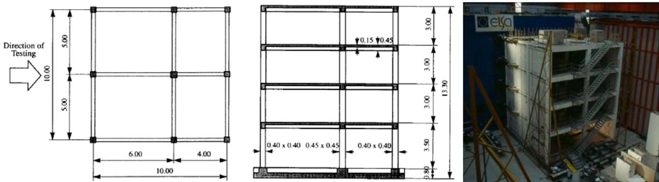
Fig. 1. Plan and elevation view of the bare and infilled RC structure.
