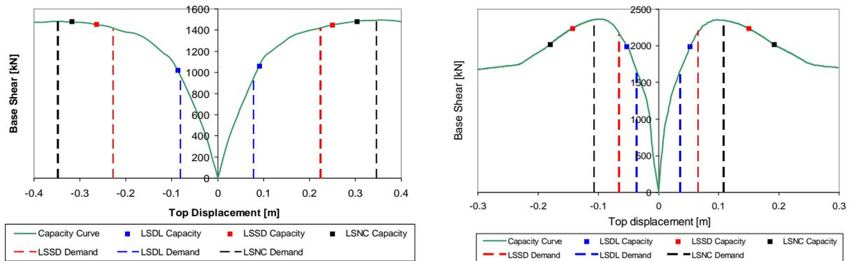
Fig. 4. Displacement capacity and demand for the bare (left) and infilled (right) structures at the different limit states.
