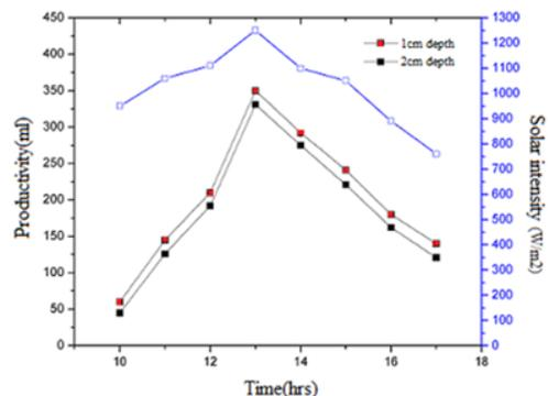
Fig. 12. productivity of finned distiller with mild steel billets
