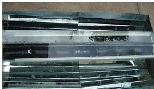
Fig. 3. Solar distiller with finned basin
