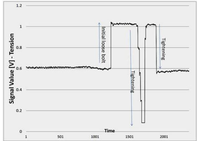
Fig. 3. Measured bolt tension.
