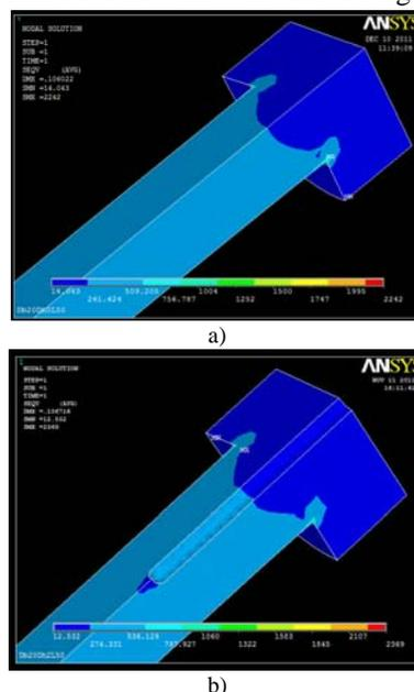
Fig. 1. Von Mises stress distribution (a) without hole and (b) with added hole to the bolt.
