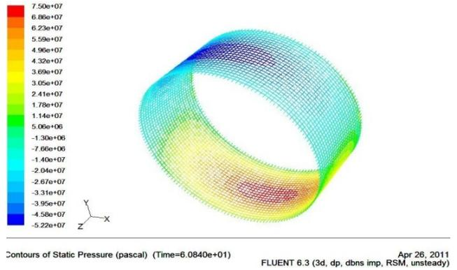
Fig. 4. Countors of Static pressure for L/D=0.5
