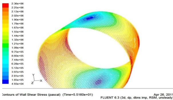
Fig. 9. Contours of Wall Shear Stress for L/D=1
