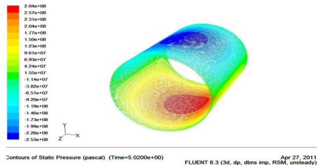
Fig. 6. Countors of Static pressure for L/D=1.5
