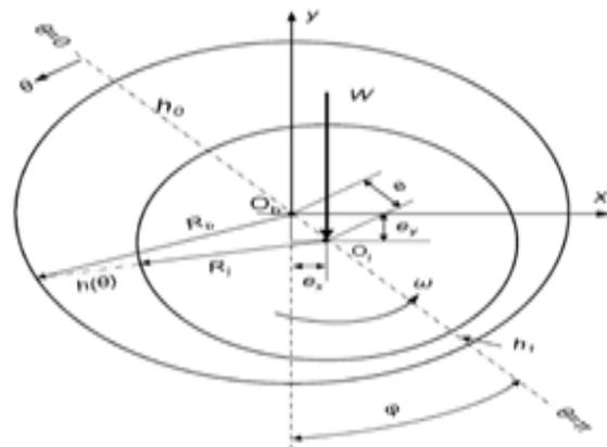
Fig. 1. Schematic diagram of Journal Bearing
