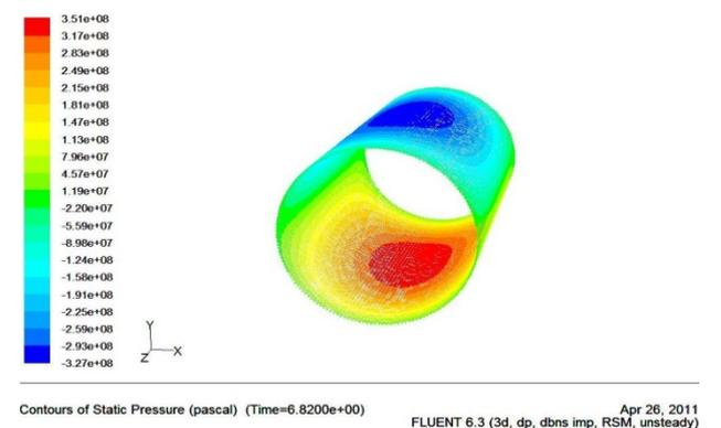
Fig. 7. Countors of Static pressure for L/D=2
