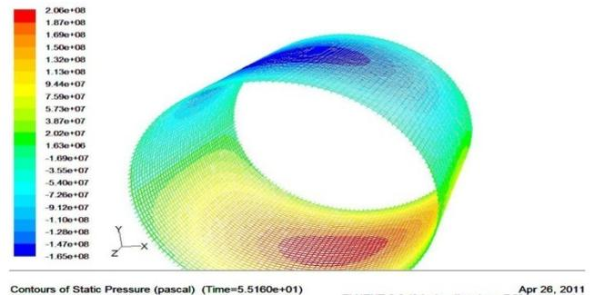
Fig. 5. Countors of Static pressure for L/D=1
