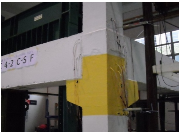
Fig. 3. SFRC in concrete at beam-column joint with corbels painted with yellow which is ready for instrumentation.
