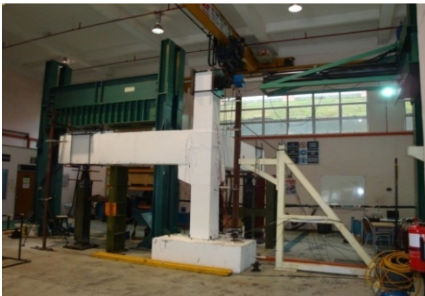
Fig. 2. Full scale beam-column joint subassembly is ready for testing
