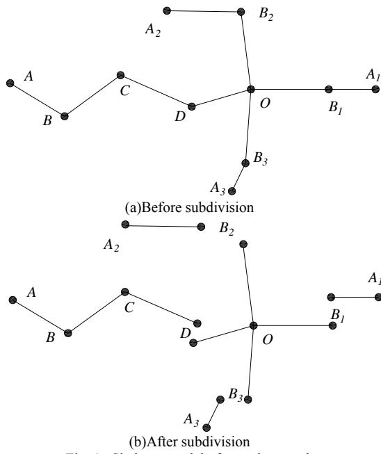
Fig. 1. Skeleton model of tunnel network
