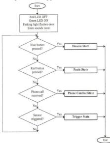
Fig. 18. The program in the arm state
