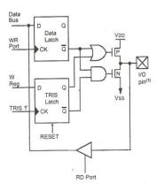
Fig. 4. Equivalent Circuit of I/O
