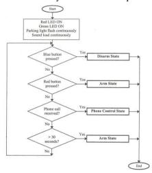
Fig. 19. The program logic in the panic state
