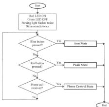
Fig. 17. The program logic in disarm state
