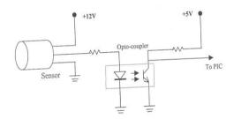
Fig. 11. Connection between PIC and sensor
