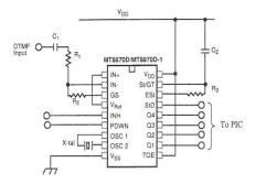
Fig. 14. DTMF decoder circuit used in PIC-mobile transceiver interface unit
