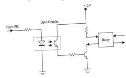
Fig. 10. Switching circuit used in PIC-car accessories interface unit
