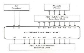
Fig. 7. PIC Based MCCS Schematic Diagram
