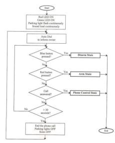
Fig. 20. Program logic in the triggered state
