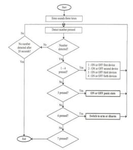
Fig. 21. The program logic in the phone control state
