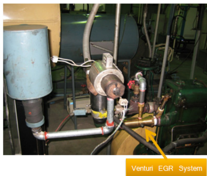
Fig. 2. Photographic view of the venturi EGR system on the intake manifold
