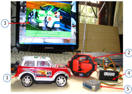
Figure 8. System Hardware of the Operation of An RC Car by Facial Commands
