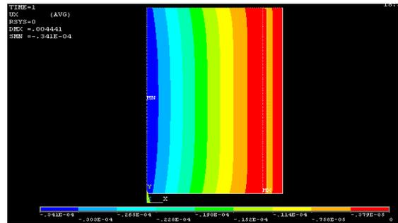
Fig.9 displacements of different sections of nuclear fuel rod
