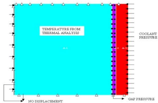
Fig.5 boundary conditions and loads for structural analysis
