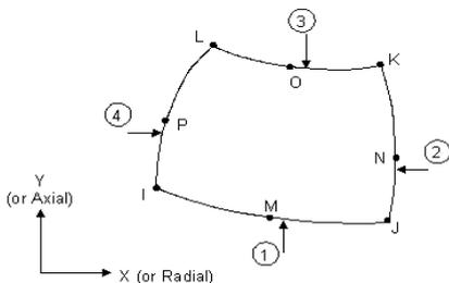
Fig.2 PLANE82 Geometry
