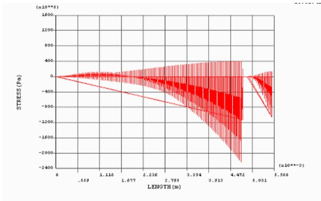
Fig. 7 stress distribution in fuel element
