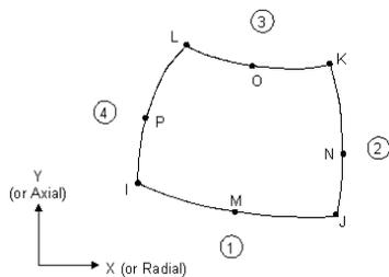
Fig.1 PLANE77 Geometry
