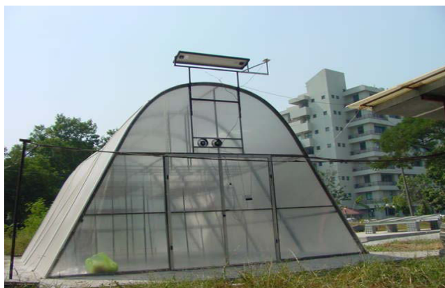
Fig. 8. Pictorial view of the greenhouse solar dryer with polycarbonate sheet.
