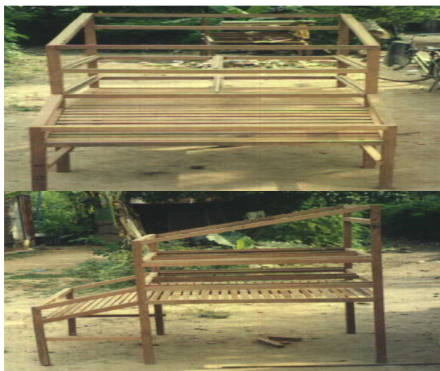
Fig. 1. Base frame of solar cabinet dryer – 1 m 2 model.
