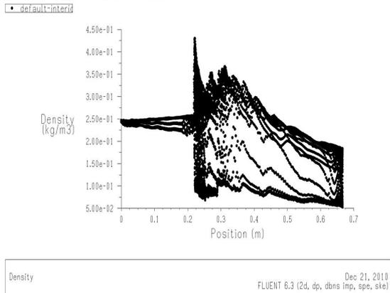
Figure 15: Density distribution at the interior
