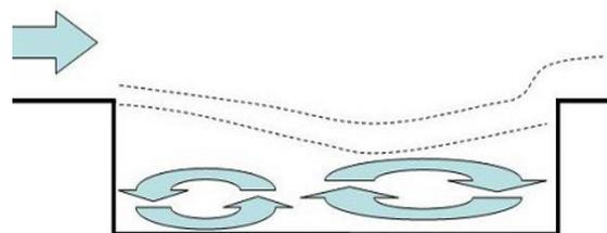
Figure 1: Rectangular cavity flame holder
